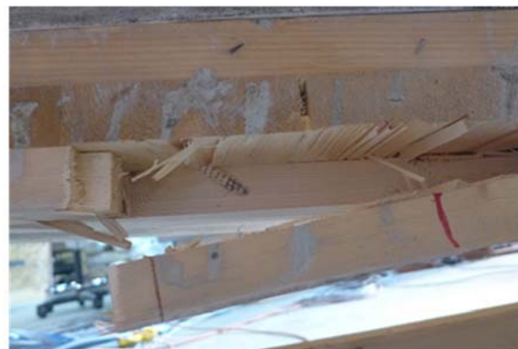
Figure 63: Series 3 panel exhibiting tensile failure prior to connector yielding or concrete crushing
