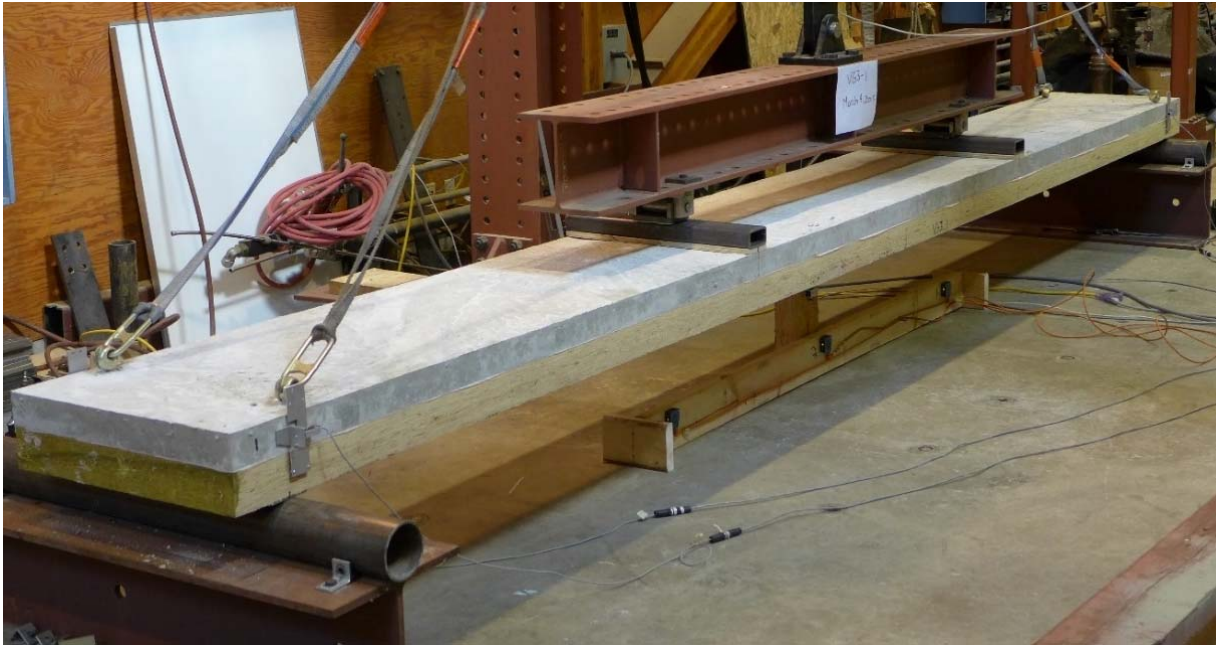
Figure 16: Photo of full-scale bending test
