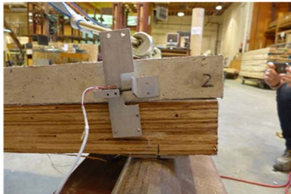
Figure 65: Series 7 panel with HBV connector prior to (left) and after yielding (right)
