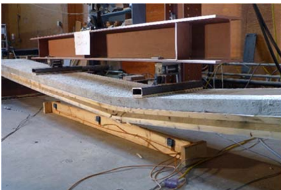
Figure 63: Series 3 panel exhibiting tensile failure prior to connector yielding or concrete crushing
