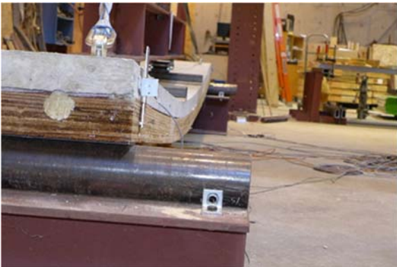
Figure 65: Series 7 panel with HBV connector prior to (left) and after yielding (right)
