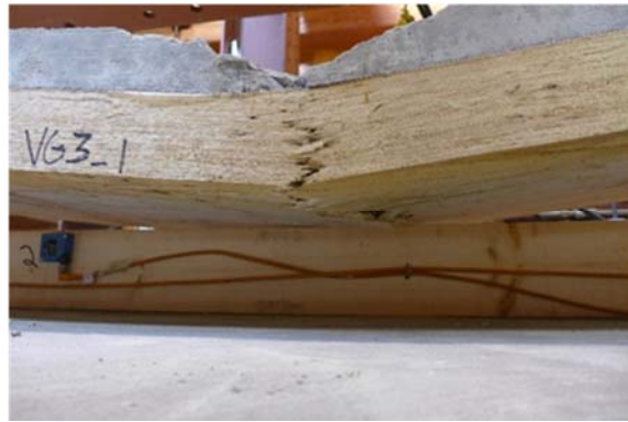
Figure 61: Series 1 Panel failing due to concrete crushing and timber tensile fracture
