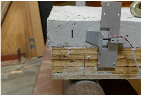
Figure 62: Series 2 panel failing by screw withdrawal followed by tensile failure of timber
