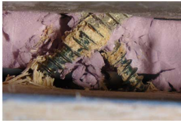
Figure 64: Series 4 panel failing by screw withdrawal through 25mm rigid insulation
