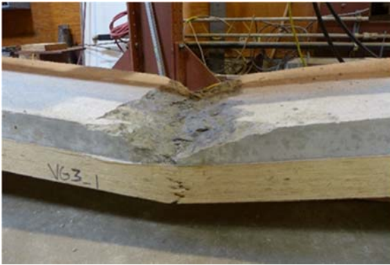
Figure 61: Series 1 Panel failing due to concrete crushing and timber tensile fracture
