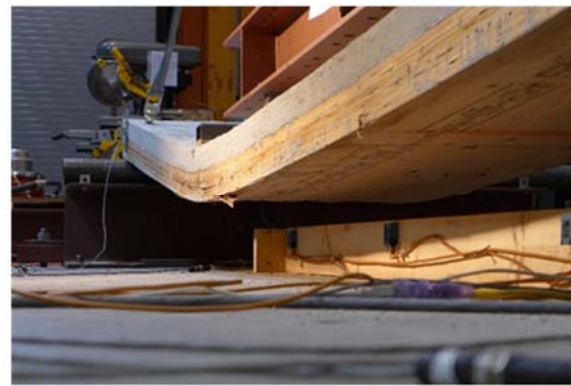
Figure 62: Series 2 panel failing by screw withdrawal followed by tensile failure of timber
